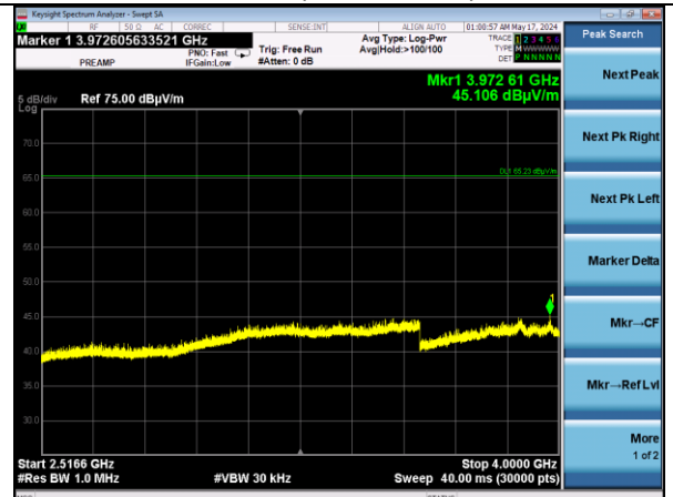
802.11b | Channel 1 | 1 Mbps | 2510.3-4000 MHz | Horizontal | Z Plane
