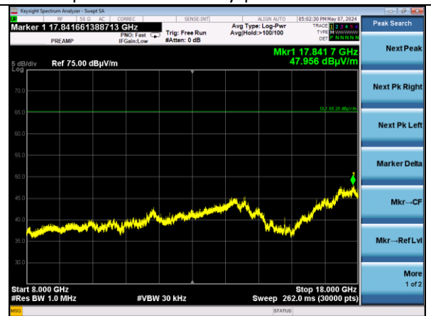
802.11a | Channel 52 | 6 Mbps | 8000-18000 MHz | Horizontal Polarity | Z orientation
