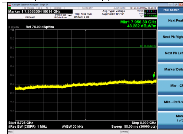
802.11ac | Channel 140 | MCS0 | 5725-8000 MHz | Horizontal Polarity | Z orientation
